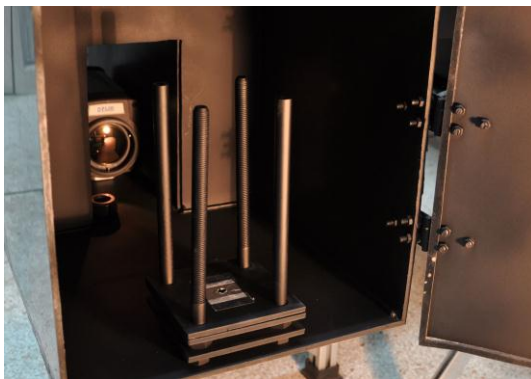
Fig. 1 The specimen holder and the thermographic camera were installed in the environmental controlling box.
