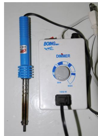
Fig. 3 A soldering iron and a dimmer are used to heat a specimen up.
