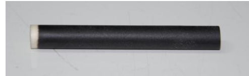
Fig. 2 Alumina rod coated with flat black spray paint is used as a specimen.
